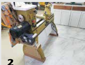
2 A vinyl tile top layer, with chamfered base molding around the lathe's legs, is easy to sweep.
